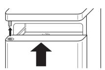
**14.** Slide the centre door bearing into the bottom left of the fridge compartment door and fasten to the housing.
